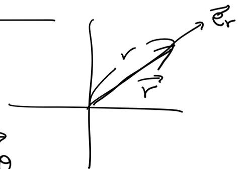
$$\vec{v} = \frac{d\vec{r}}{dt} = \dot{\vec{r}} = \dot{r} \vec{e}_r + r \dot{\vec{e}}_r = \dot{r} \vec{e}_r + r \dot{\theta} \vec{e}_\theta$$
