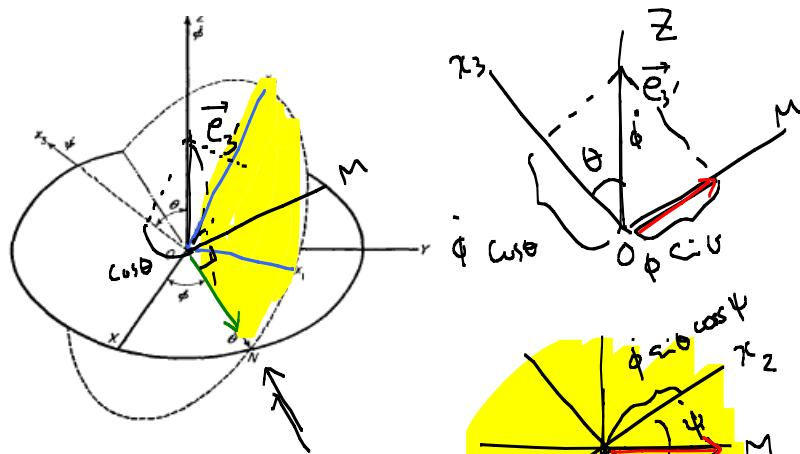
$$\begin{aligned}\vec{\Omega}_1 &= \dot{\phi} \vec{e}'_3 \\ \vec{\Omega}_2 &= \dot{\theta} \vec{e}'_1 \\ \vec{\Omega}_3 &= \dot{\psi} \vec{e}''_3\end{aligned}\quad \left. \right\} \vec{\Omega} = \vec{\Omega}_1 + \vec{\Omega}_2 + \vec{\Omega}_3$$
