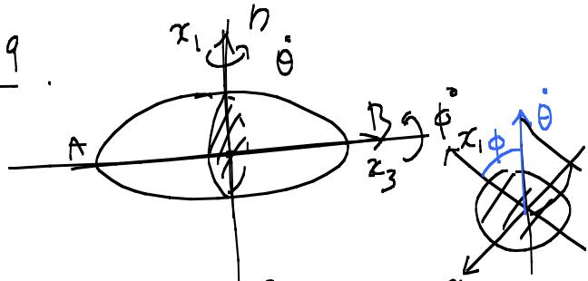
$$\vec{\Omega} = \underbrace{\dot{\theta} \vec{e}_1}_{\omega_1} + \underbrace{\dot{\phi} \vec{e}_3}_{\omega_3} + \underbrace{\vec{e}_2 \dot{\theta} \sin \phi}_{\omega_2}$$
