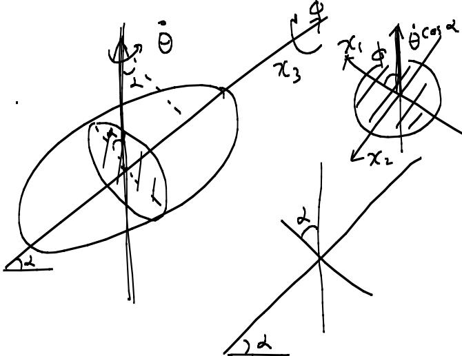
$$\vec{\Omega} = \vec{e}_3 (\dot{\phi} + \dot{\theta} \sin \alpha) + \vec{e}_1 (\dot{\theta} \cos \alpha \cos \phi) + \vec{e}_2 (-\dot{\theta} \cos \alpha \sin \phi)$$
