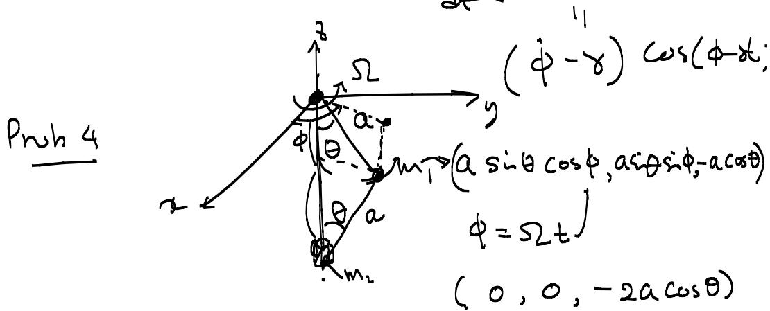
$$\vec{v}_1 = a \left( \dot{\theta} \cos \theta \cos \phi - \Omega \sin \theta \sin \phi, \dot{\theta} \cos \theta \sin \phi + \Omega \sin \theta \cos \phi, \dot{\theta} \sin \theta \right)$$
