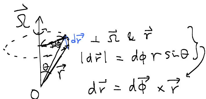
$$\vec{v}_{\text{Fixed}} = \vec{V} + \frac{d\vec{\phi}}{dt} \times \vec{r} = \vec{V} + \vec{\omega} \times \vec{r}$$
