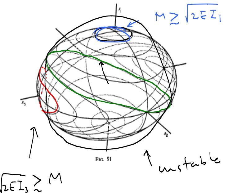
$$2E I_3 = (I_1^2 \Omega_1^2 + I_2^2 \Omega_2^2 + I_3^2 \Omega_3^2)$$
