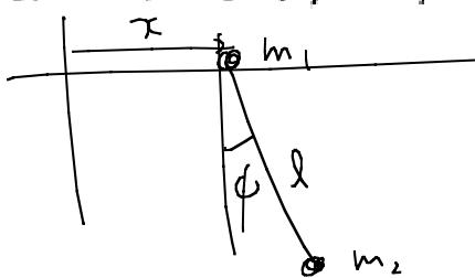
$$\frac{\partial L}{\partial x} = 0 \rightarrow \frac{\partial L}{\partial \dot{x}} = \text{const} = P_x$$
