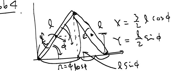
$$\begin{aligned} T &= \frac{T^{(1)}_{\text{trans}} + T^{(1)}_{\text{rot}}}{\frac{1}{2} \mu l^2 (\frac{1}{2} \dot{\phi}^2) + \frac{1}{2} \frac{T}{I_2} \dot{\phi}^2} \\ &= \frac{1}{2} \mu \left( \frac{l}{2} \dot{\phi} \right)^2 + \frac{1}{2} \frac{T}{I_2} \dot{\phi}^2 \\ &\quad \underbrace{\frac{1}{2} \left[ \mu l^2 \left( \frac{1}{4} + \frac{1}{12} \right) \dot{\phi}^2 \right]}_{\frac{1}{3} T} = I \ddot{\phi} \end{aligned}$$
