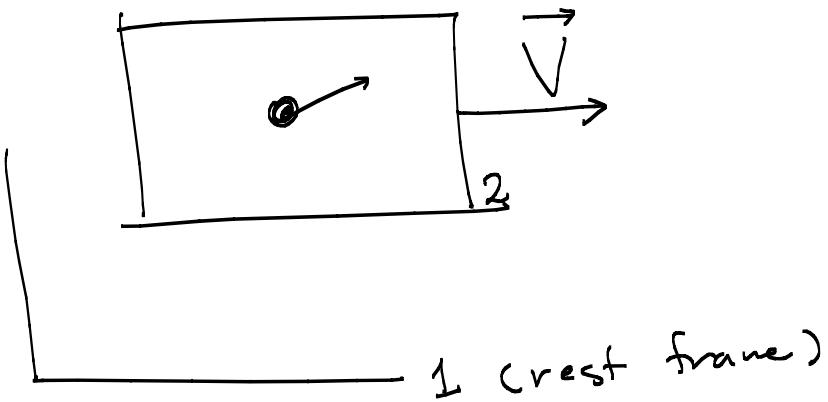
If  $\vec{F} = 0$  in rest frame,  $\vec{F} = 0$  in a constant moving frame. (inertial frame)
