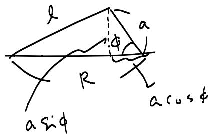
$$\begin{aligned} l^2 &= a^2 \sin^2 \phi + (R - a \cos \phi)^2 \\ &= R^2 + a^2 - 2R a \cos \phi \end{aligned}$$
